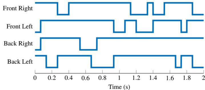
**Fig. 4** Contact mode sequence for each foot from LittleDog step-climbing example.
