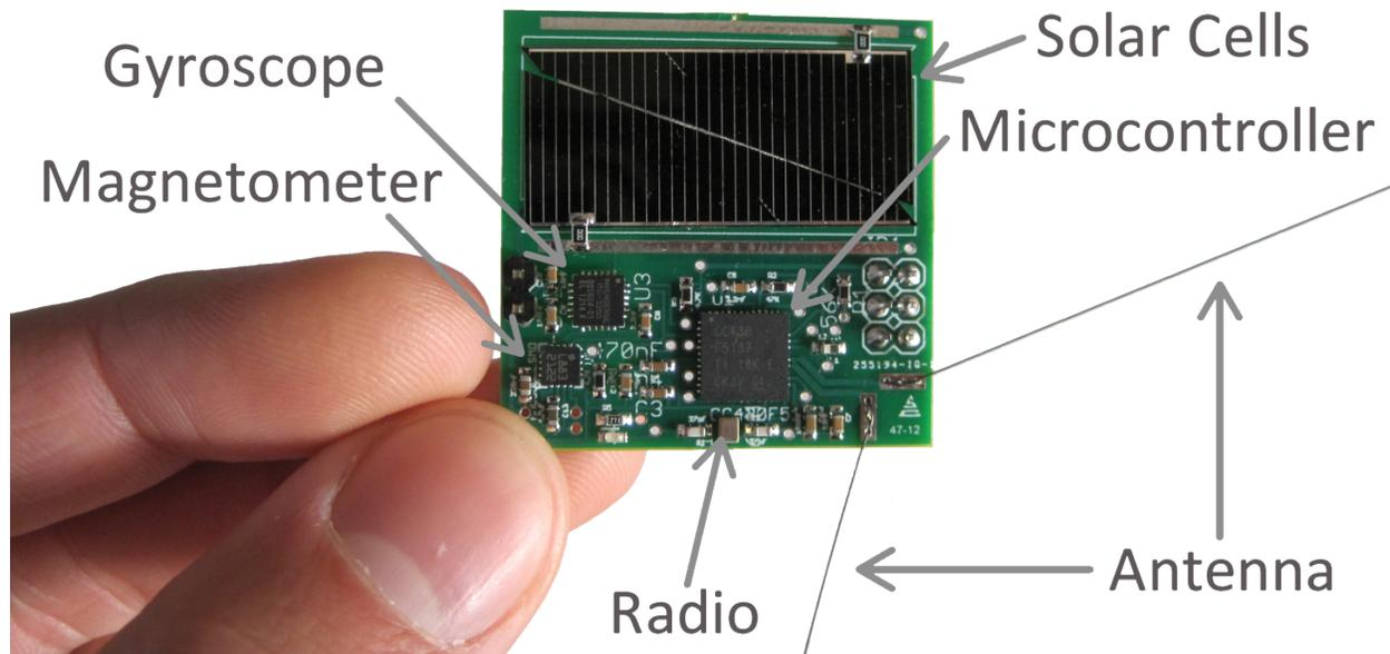
Figure 3: Sprite ChipSat
