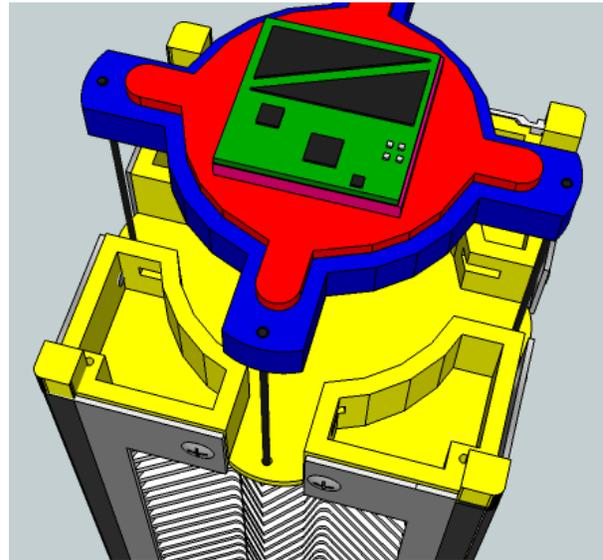
**Figure 9: Deployer Locking Mechanism**
