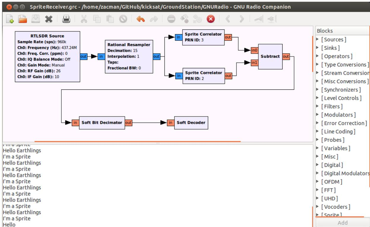
**Figure 5: GNU Radio Receiver**
