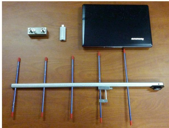
**Figure 4: Ground Station Hardware**
